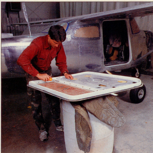
An acid etch wash (above) neutralizes surface corrosion and prepares the aluminum to receive the alodine conversion coating. New windows go in after the danger of stripper damage is past.
