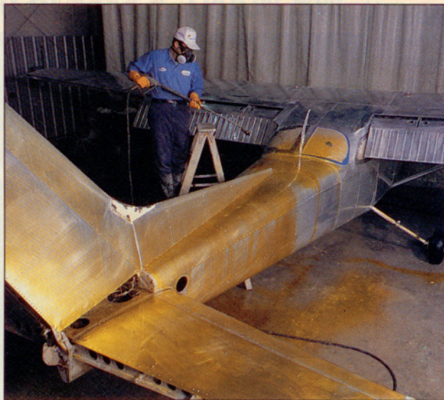
The gold-colored alodine conversion coating fends off corrosion and helps adhere the primer to the surface.
