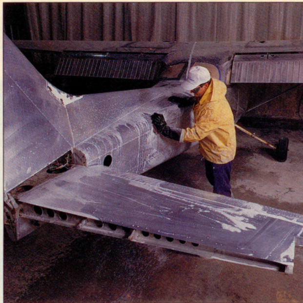
An acid etch wash (above) neutralizes surface corrosion and prepares the aluminum to receive the alodine conversion coating. New windows go in after the danger of stripper damage is past.
